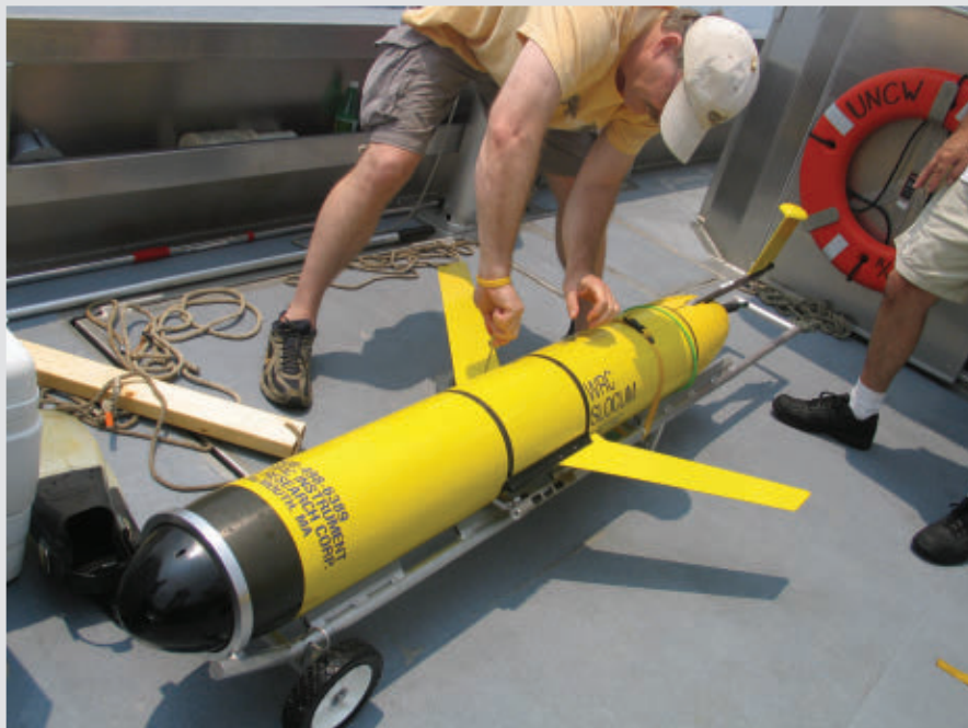
Navy researchers are counting on sea glider UUV technology for long-duration persistent surveillance of the ocean's depths.
