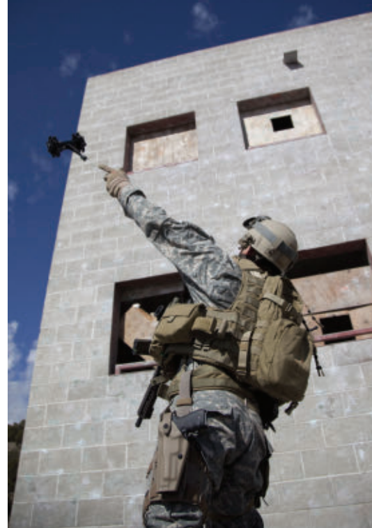
Equipped with video, audio and infrared sensors, the ReconRobotics Throwbot XT can be deployed in three seconds and thrown as far as 120 feet.
