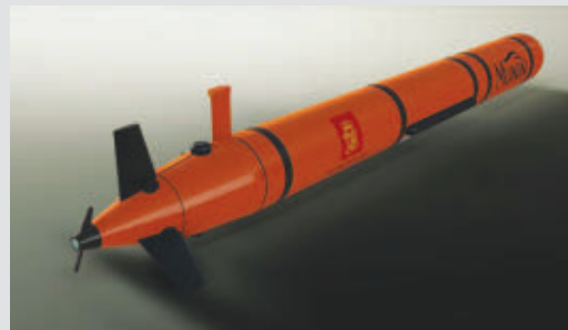
The Kongsberg MUNIN unmanned submersible, shown above, is for offshore persistent surveillance.
